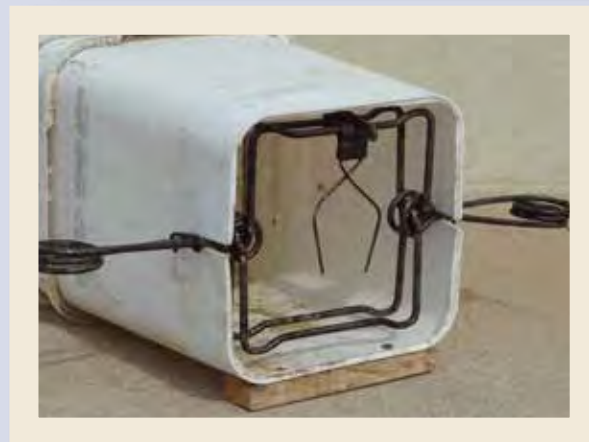
Figure 4. Typical trigger configurations; placement is top center and shape is inverted "U" or "V."
