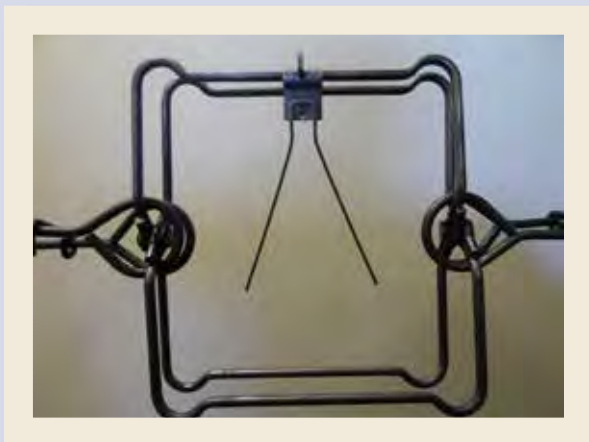
Figure 4. Typical trigger configurations; placement is top center and shape is inverted "U" or "V."
