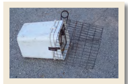
Figure 7. Recessed bucket set with wire enclosure
